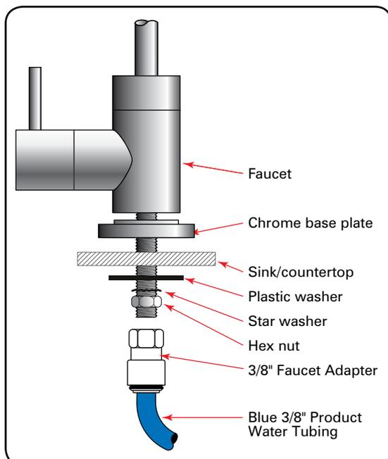
Take length of 3/8" blue tube and make sure it has a fresh cut and is free of foreign materials and any scratches on the outside surface. Install the tubing into the push in type fitting at the base of the faucet. Make certain that it is inserted all the way in; once inserted give it a slight pull to make sure it is locked into the fitting.
