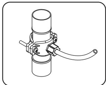
4. Attach 1/4" black tube by slipping the tube through the black compression nut and hand tighten the nut on to the saddle valve.
